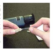
4) Reinsert the patchcord and test for signal strength.
